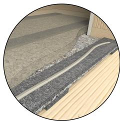
Where cutting of panels leads to removal of inbuilt isolation strip, add a continuous length of 5mm isolation material to the inside edge of panel, using a generous amount of construction adhesive.
